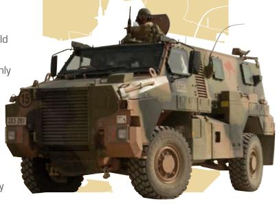
range of battlefield and peacekeeping applications. Roof mountings to fix a remote weapons station, light cannon and smoke grenades transform Bushmaster into a highly effective Armed Personnel Carrier.
