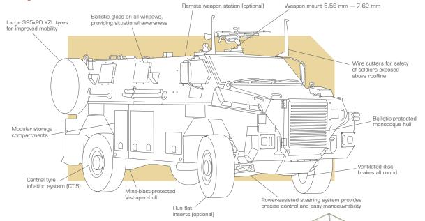
Bushmaster's integrated high hardness and transparent armour, specialist welding and the shaping of its monocoque hull, protect troops and mechanical components from land mines and other blast weapons as well as small arms and artillery fragments.
